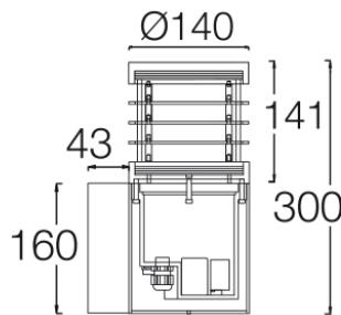
Wall-mounted fixture with 360° light emission, radial beam. Cylindrical design with a diameter of 140mm.
