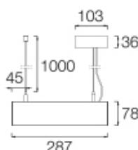
**Luminaire luminous flux:** 1283lm
