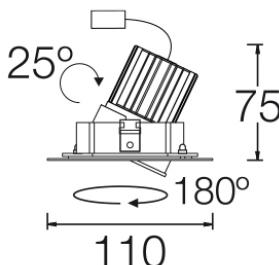
**Luminaire luminous flux:** 590lm
