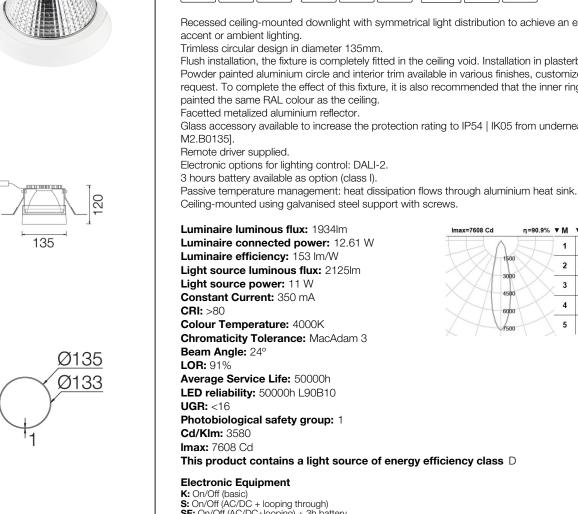
SE: On/Off (AC/DC+looping) + 3h battery D: DALI-2/switchDIM/corridorFUNCTION DE: DALI-2/switchDIM/corridorFUNCTION + Battery 3h B: Bluetooth-Casambi
