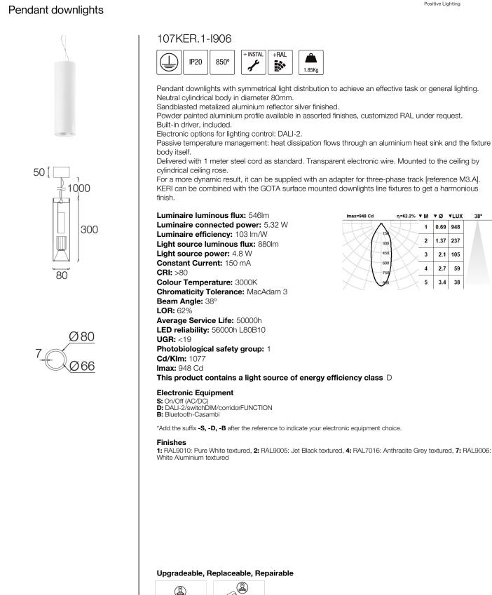
For a more dynamic result, it can be supplied with an adapter for three-phase track [reference M3.A]. KERI can be combined with the GOTA surface mounted downlights line fixtures to get a harmonious
