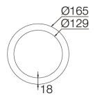
Luminaire luminous flux: 1615lm Luminaire connected power: 12.61 W Luminaire efficiency: 128 lm/W Light source luminous flux: 1815lm Light source power: 11 W Constant Current: 350 mA **CRI:** >90 Colour Temperature: 4000K Chromaticity Tolerance: MacAdam 3 Beam Angle: 40° LOR: 89% Average Service Life: 50000h LED reliability: 50000h L90B10 **UGR:** 16 Photobiological safety group: 1 Cd/Klm: 1631 Imax: 2960 Cd
