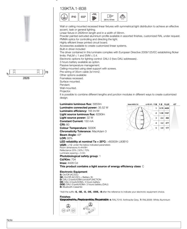
LED technology and performance data are constantly changing. Current details should therefore be checked with ROVASI in order to ensure that it is still the most up to date reference. Updated data will be supplied on request. [Last revised on 06.06.2025]
