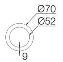
Luminaire luminous flux: 940lm Luminaire connected power: 11.27 W Luminaire efficiency: 83 lm/W Light source luminous flux: 940lm Light source power: 10 W Constant Current: 300 mA **CRI:** >90 Colour Temperature: 3000K Chromaticity Tolerance: MacAdam 3 Beam Angle: 36° LOR: 100% Average Service Life: 50000h LED reliability: >50000h L90B10 **UGR:** <19 Photobiological safety group: 1 Cd/Klm: 2063 Imax: 1930 Cd
